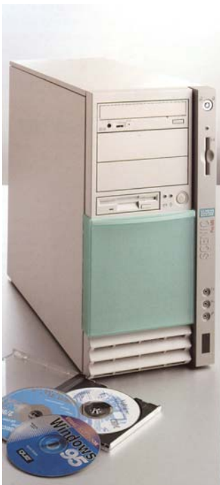
计算机主机外壳 / Computer housing (Novodur ABS)
