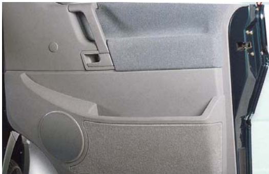
车门内衬 / Door lining (Novodur ABS)
